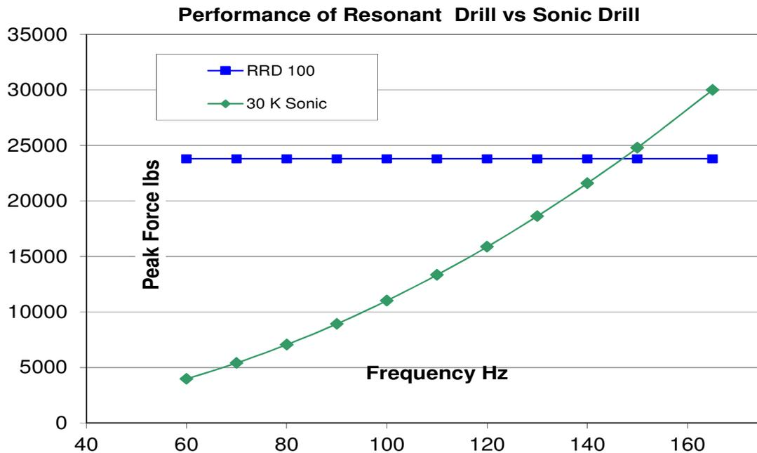
**Figure 1. Frequency vs. peak force for typical Resonant and Sonic Drills**
